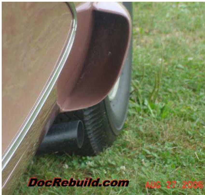
Note the drivers side brake duct and exhaust dump.
