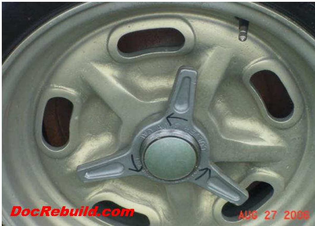
Note the left hand threaded spinner and number of threads visible of these Halibrand KO adaptors. I love those arrows.
