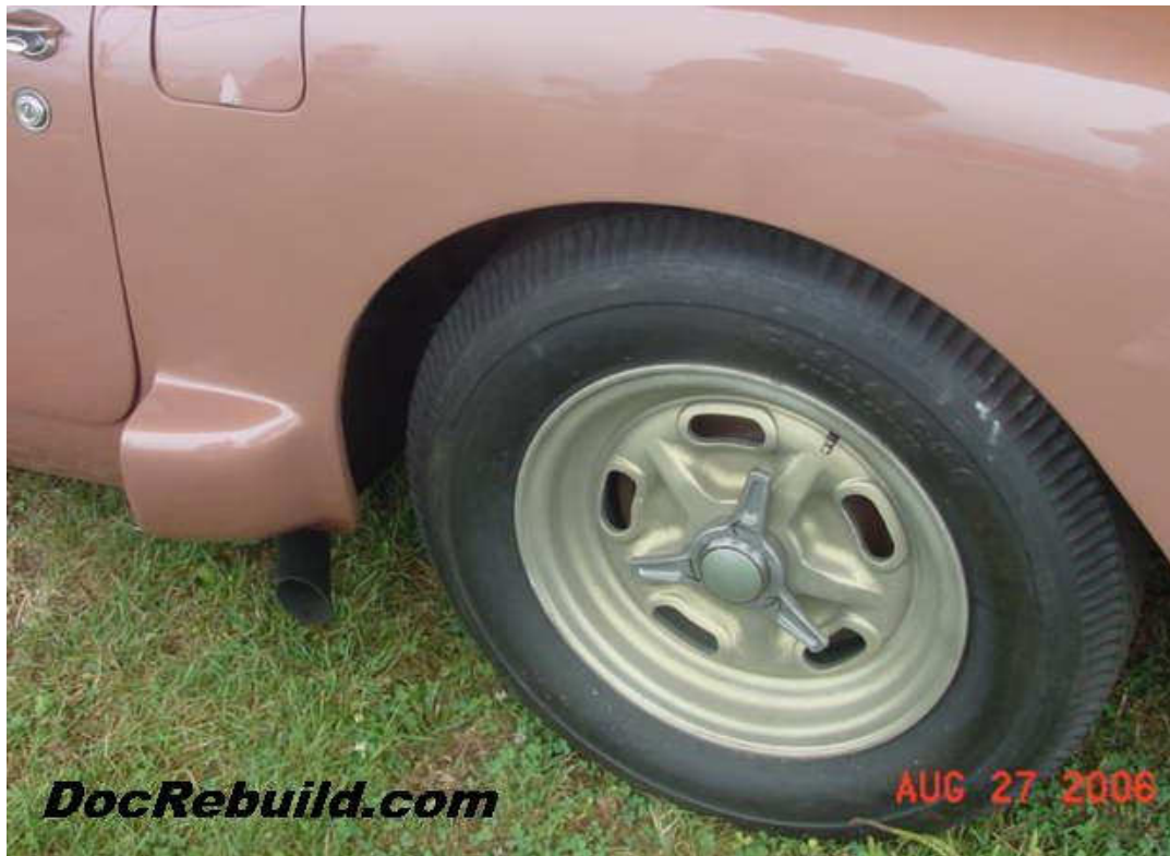
These brake cooling duct scoops are the tell tale identifier of all these SR-1 models.
